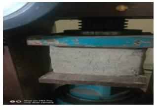
Fig 3: Compressive strength test
